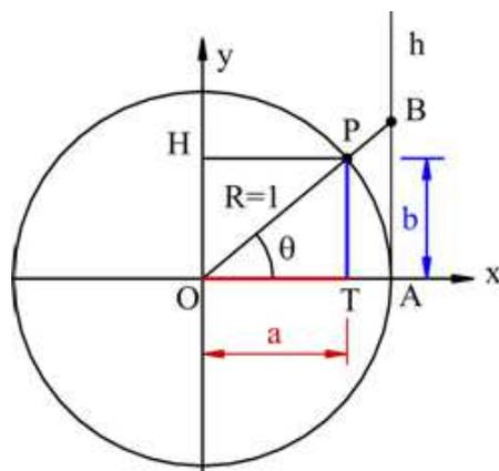
$$\frac{\overline{PT}}{\overline{OT}} = \frac{\overline{AB}}{\overline{OA}} \Rightarrow \frac{b}{a} = \frac{\overline{AB}}{R} = \operatorname{tg}\theta$$
